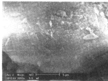
Fig. 1 Scanning electron microscopy (SEM) of the illite (the scale was 5 \mu\text{m} )
