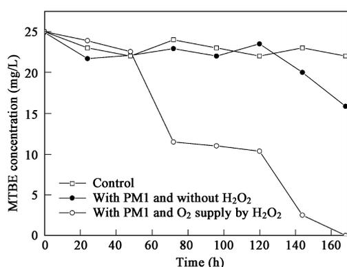
Fig. 2 Methyl *tert*-butyl ether (MTBE) degradation by PM1 in the closed system seeded with 1 ml of inoculum (cell concentration: 10<sup>7</sup> cfu/ml) into 5 ml medium.
