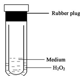
Fig. 1 Diagram of closed system for MTBE degradation by PM1.
