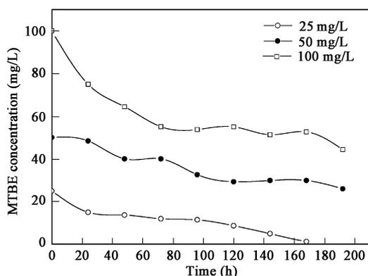
Fig. 4 Effect of initial concentration on MTBE degradation in closed system with 1 ml of inoculum ( $1.5 \times 10^7$  cfu/ml) added into 5 ml medium.
