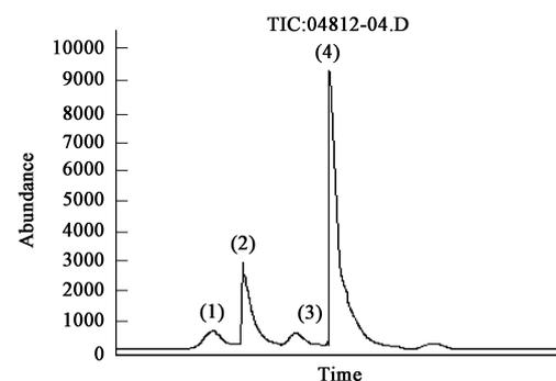
Fig. 6 P&T GC/MS spectra of the broth of MTBE degradation by PM1 in closed system. (1) isopropanol; (2) acetone; (3) TBA; (4) MTBE.
