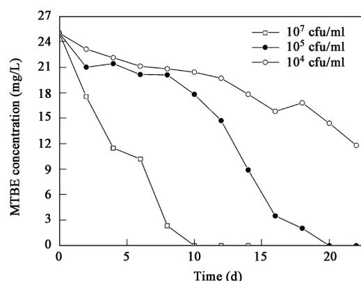
Fig. 3 Effect of cell concentration of inoculum on MTBE degradation by PM1 in closed system with 1 ml of inoculum added into 5 ml medium.
