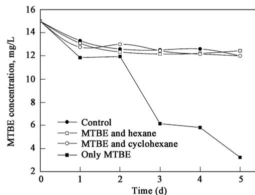
Fig. 5 Effect of co-metabolic substances on MTBE degradation by PM1 in closed system.
