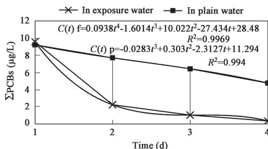
Fig. 1 PCBs measured concentration and curve of analog approach in the water.
