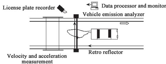
Fig. 1 Remote sensing system of vehicle emission based on tunable diode laser technique.
