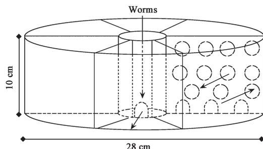
Fig. 1 Test container of the avoidance response test (Schaefer, 2004). Arrow presents free migration possibility.
