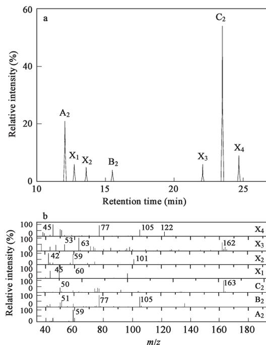
Fig. 4 GC chromatogram from the TiO<sub>2</sub>-assisted (TiO<sub>2</sub> nanostripe) photodegradation of RhB after visible light irradiation of 41 h (a) and mass spectra of the species observed in the GC shown in Fig.4a (b).
