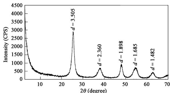
Fig. 3 XRD spectrum of the anatase type nano  $\text{TiO}_2$ .
