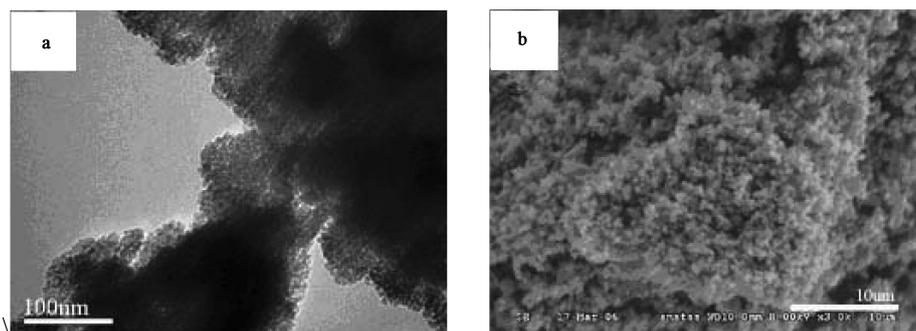
Fig. 1 Nano size TiO<sub>2</sub> morphology by TEM (a) and SEM (b).
