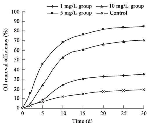
Fig. 2 Oil removal efficiency under different nitrate concentrations.
