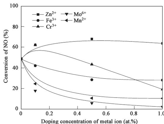
Fig. 2 NO conversion efficiency of catalysts with different ion doping. 125 W Hg-arc lamp; relative humidity: 80%; O<sub>2</sub> concentration: 21%; EBRT: 10 s.
