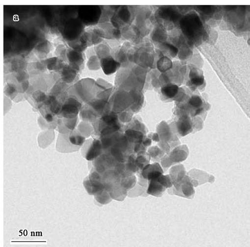
the Scherrer equation, ranged from 20 to 25 nm. And the rutile crystal sizes were within the range between 50 and 60 nm. It was found that the crystal size of doped catalysts had little change with the pure Degussa P25 particles.
