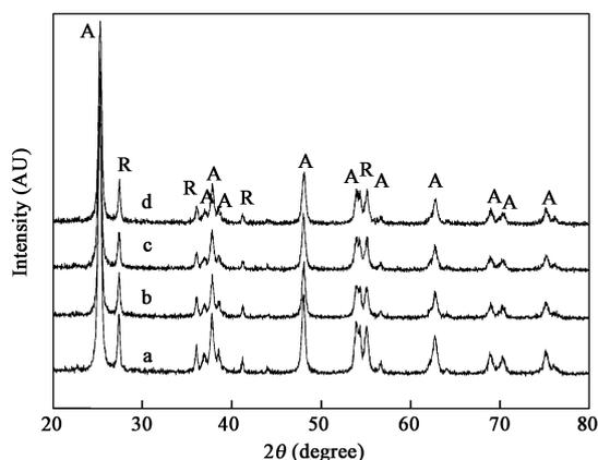
Fig. 3 XRD patterns of  $Fe^{3+}$  doped  $TiO_2$  catalysts with different doping concentration. (a) Degussa P25; (b) 0.01 at.%  $Fe^{3+}$ ; (c) 0.05 at.%  $Fe^{3+}$ ; (d) 1.0 at.%  $Fe^{3+}$ .
