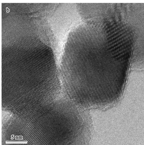
Fig. 4 TEM and HR-TEM micrographs of  $Zn^{2+}$  doped  $TiO_2$  particles. (a) TEM of 0.5 at.%  $Zn^{2+}$  doped  $TiO_2$  particles; (b) HR-TEM of 0.5 at.%  $Zn^{2+}$  doped  $TiO_2$  particles.
