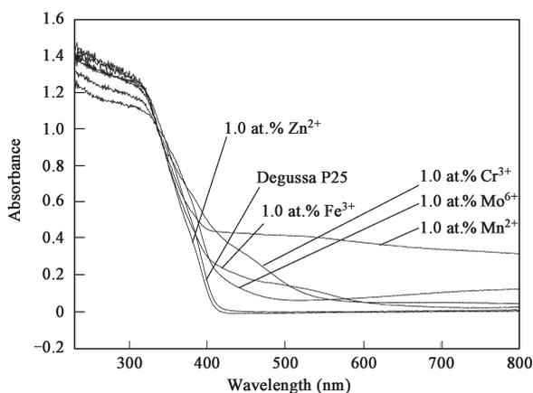
Fig. 6 UV-Vis absorbance spectra for the ion doped titania powder.
