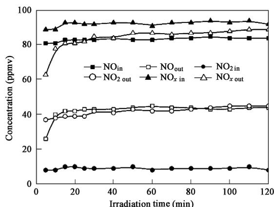
Fig. 1 Photocatalytic behavior of nitric oxide. 125 W Hg-arc lamp; relative humidity: 60%; EBRT: 10 s; O<sub>2</sub> concentration: 21%; catalyst: Degussa P25.
