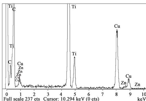
Fig. 5 EDS spectra of 0.5 at.% Zn<sup>2+</sup> doped TiO<sub>2</sub> particles.
