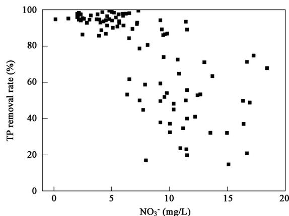
Fig. 6 Scatter of TP removal rate to effluent  $\text{NO}_3^-$ .
