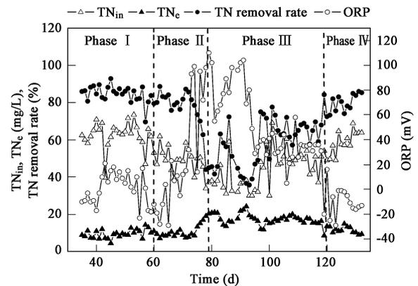
**Fig. 2** Influent and effluent TN, TN removal rate, and ORP profiles.
