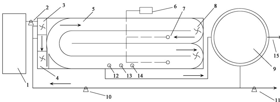
**Fig. 1** Schematic diagram of the oxidation ditch system. (1) water tank; (2) influent pump; (3) anaerobic zone; (4) anoxic zone; (5) aerobic zone of OD; (6) air pump; (7) air diffuser; (8) mixer; (9) secondary clarifier; (10) returned activated sludge pump; (11) wasted activated sludge pump; (12) DO probe; (13) ORP probe; (14) pH probe; (15) effluent.
