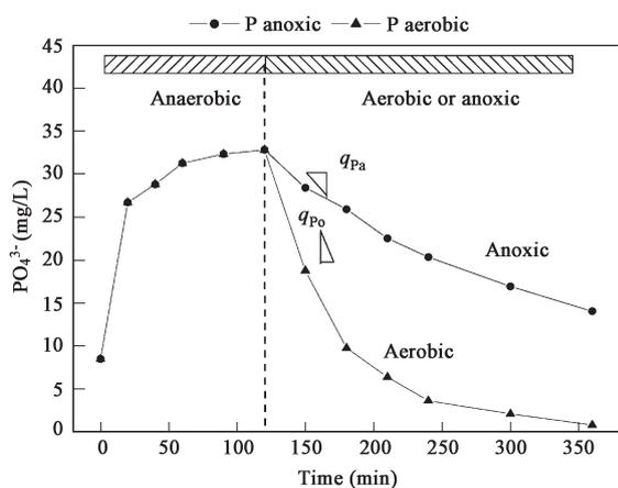
Fig. 7 Phosphorus release and uptake under anaerobic-aerobic and anaerobic-anoxic conditions.
