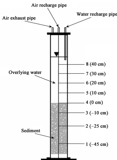
Fig. 1 Set up of column experiment. The numbers in the figure indicate the locations of suction cups.
