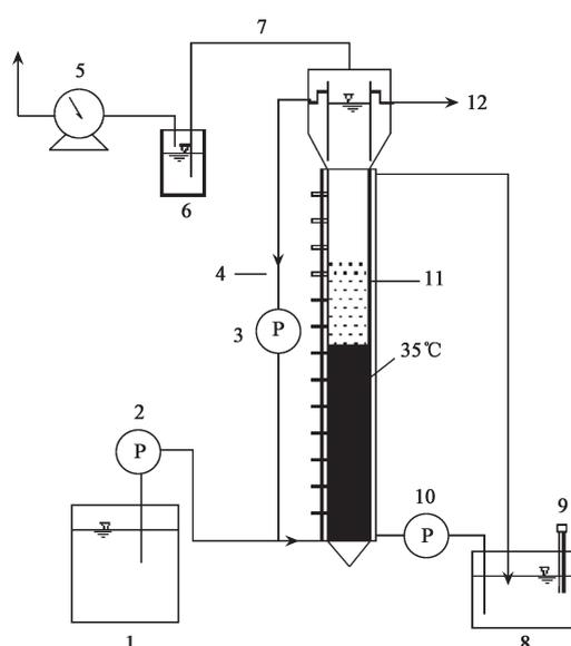
**Fig. 1** Schematic diagram of anaerobic expanded granular sludge bed reactor treating POME. (1) feed tank; (2) peristaltic pump; (3) recirculation pump; (4) sampling ports; (5) gas meter; (6) gas seal; (7) gas; (8) water bath; (9) heater; (10) centrifuge pump; (11) water jacket; (12) effluent.
