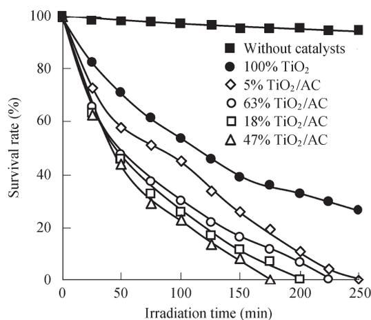
**Fig. 2** Time course of changes in the survival rate of *E. coli* caused by photocatalysis with 2 g/L of TiO<sub>2</sub>/AC catalyst or without catalysts. *E. coli* content is 1 × 10<sup>7</sup> cfu/ml.
