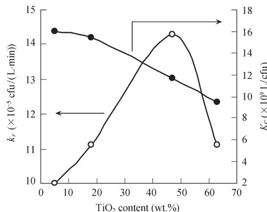
Fig. 4 Rate constant ( $k_r$ ) of *E. coli* inactivated reaction and the adsorption equilibrium constant ( $K_C$ ) of *E. coli* as a function of the  $TiO_2$  content in composite catalyst.
