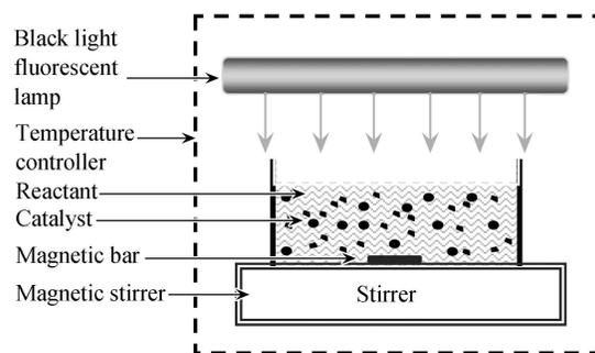
Fig. 1 Experimental apparatus for photocatalytic reaction.
