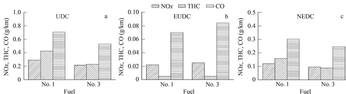
Fig. 4 Effect of hydrocarbon compositions on tailpipe emissions over UDC (a), EUDC (b), and new European driving cycle (NEDC) (c) cycles.
