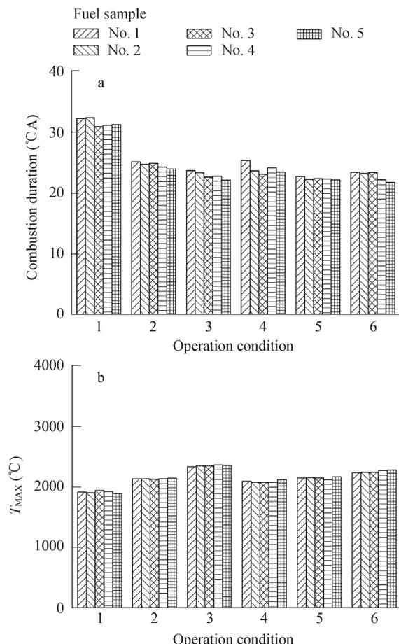
**Fig. 3** Effect of hydrocarbon compositions on combustion duration (a) and  $T_{MAX}$  (b).
