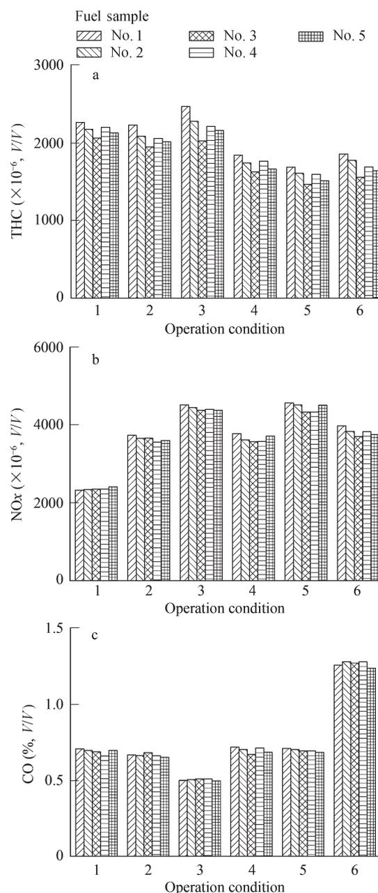
**Fig. 2** Effect of hydrocarbon compositions on engine-out THC (a), NO<sub>x</sub> (b) and CO (c) emissions.
