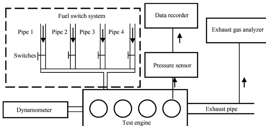
**Fig. 1** Schematic of the engine test bench.
