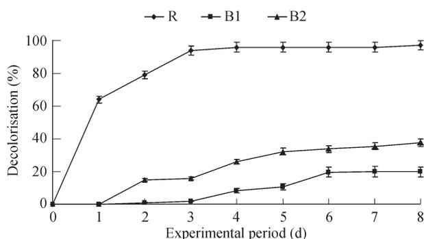
**Fig. 1** Adsorption vs. degradation by the fungus under different control conditions reactors (R, B1, B2).
