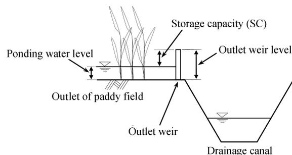
**Fig. 1** Storage capacity and outlet weir level.
