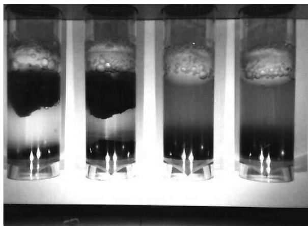
**Fig. 1** IRB-BART test indicated that the black growths on the inside wall of the AC pipe contained iron related bacteria. The two samples used in the testers on the left came from black growths attached to the inside AC pipe. The two samples on right were controls.
