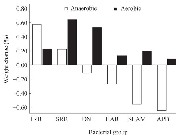
**Fig. 3** Percentage of wet weight change of AC segments after 10 days immersion in previously prepared bacterial cultures.
