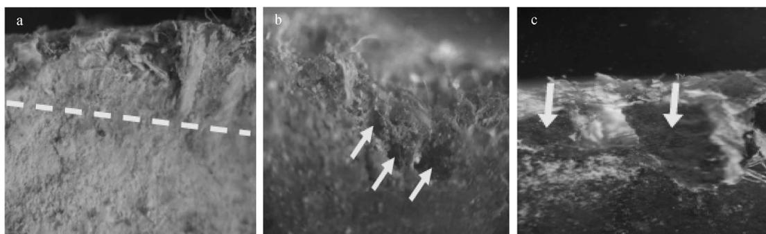
**Fig. 2** Photos of AC pipe. (a) inside wall of AC pipe is coated with a layer of patina 3–4 mm depth; (b) patina is thick fibrous films that are composed of high fibrous asbestos and some biomass forming gelatinous like materials; (c) patina tends to have yellow to brown colorations implying the presence of some iron.
