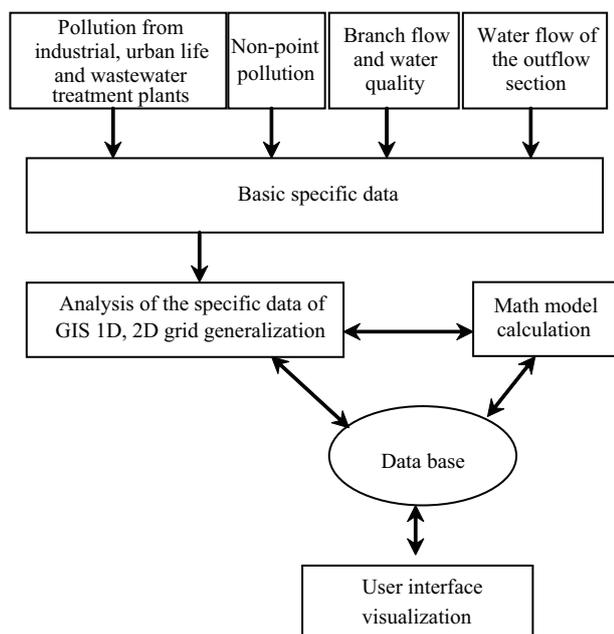
Fig. 1 Overall structure of WPMS\_ER\_TGRA.
