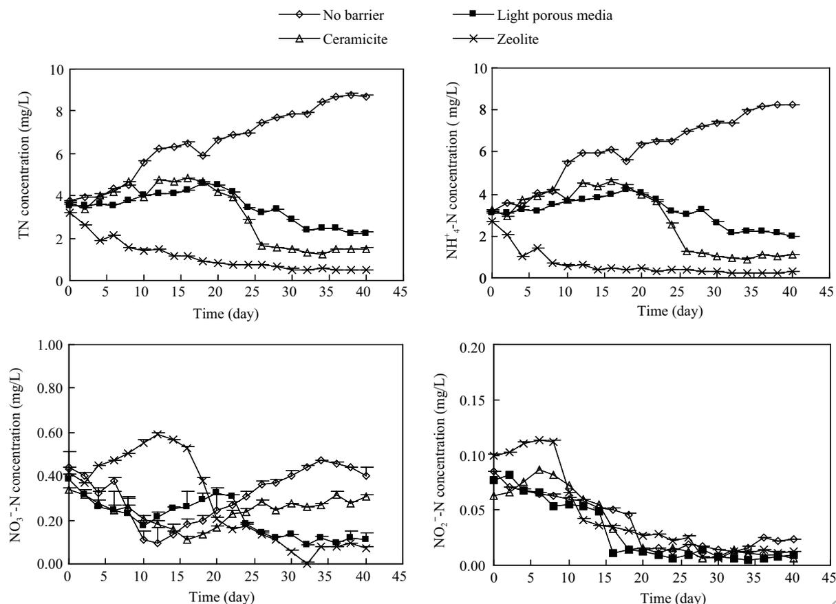
**Fig. 1** Effect of cap materials on nitrogen removal in overlying water. Condition: pH 6.5–7.5; initial ammonium concentration 3.75 mg/L; initial TN concentration 3.75 mg/L; temperature 20–25°C.
