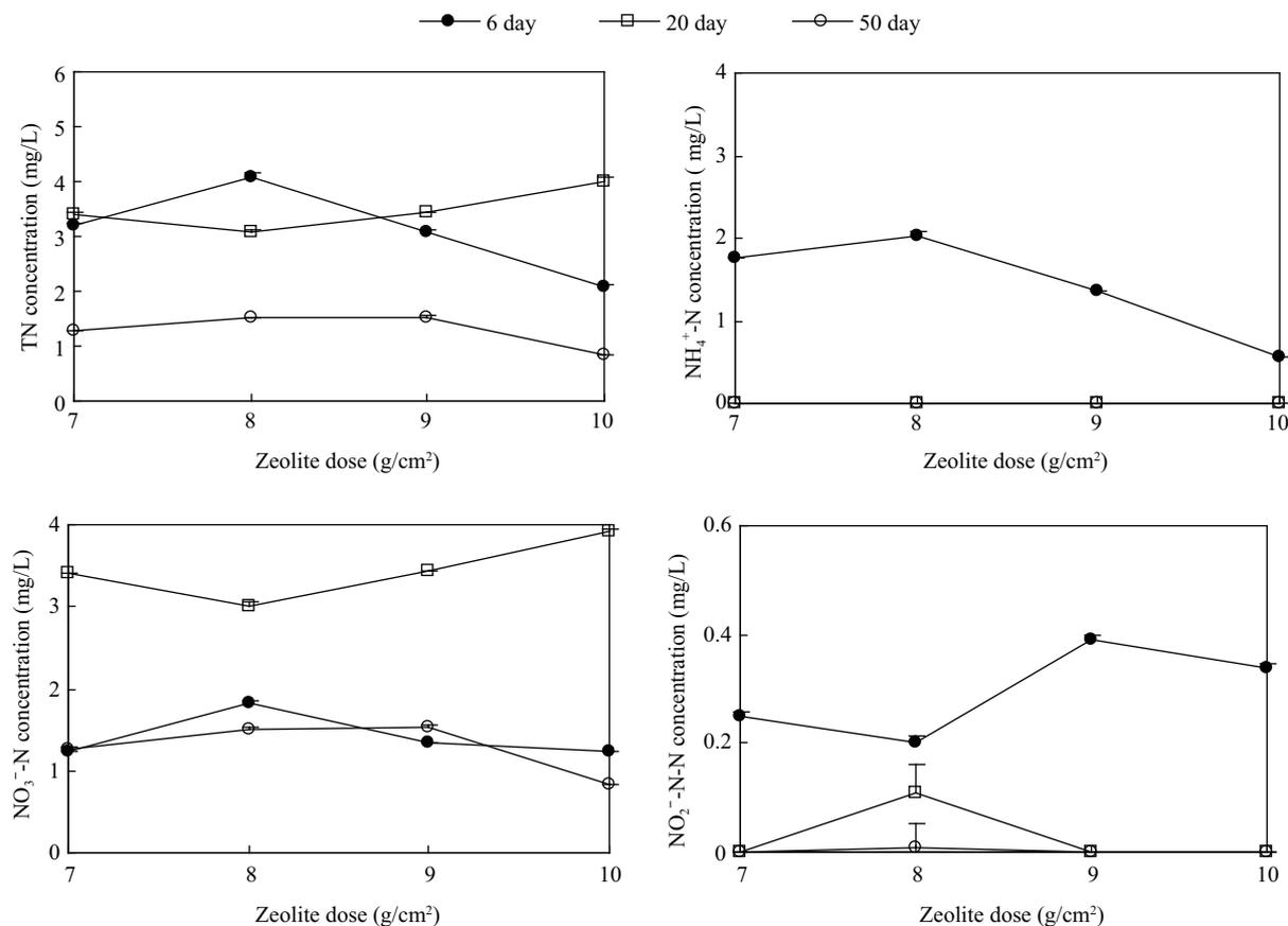
Fig. 4 Effect of bio-zeolite dose on N removal in overlying water.
