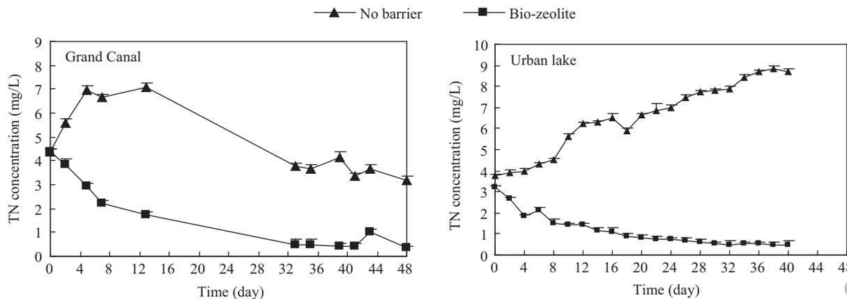
Fig. 3 Curve of TN concentration in sediments from Xi'an and Yangzhou.
