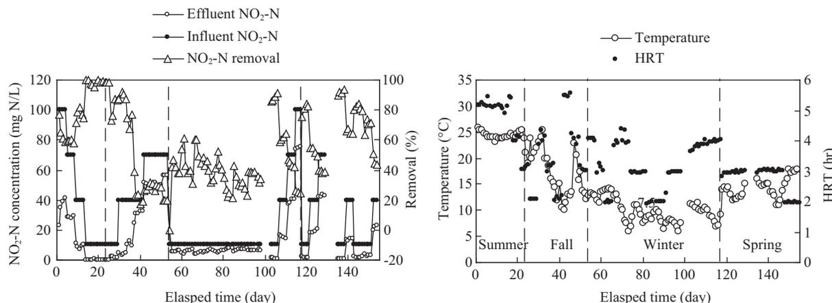
Fig. 3 Running performance of the continuous reactor treating nitrite-contaminated water.
