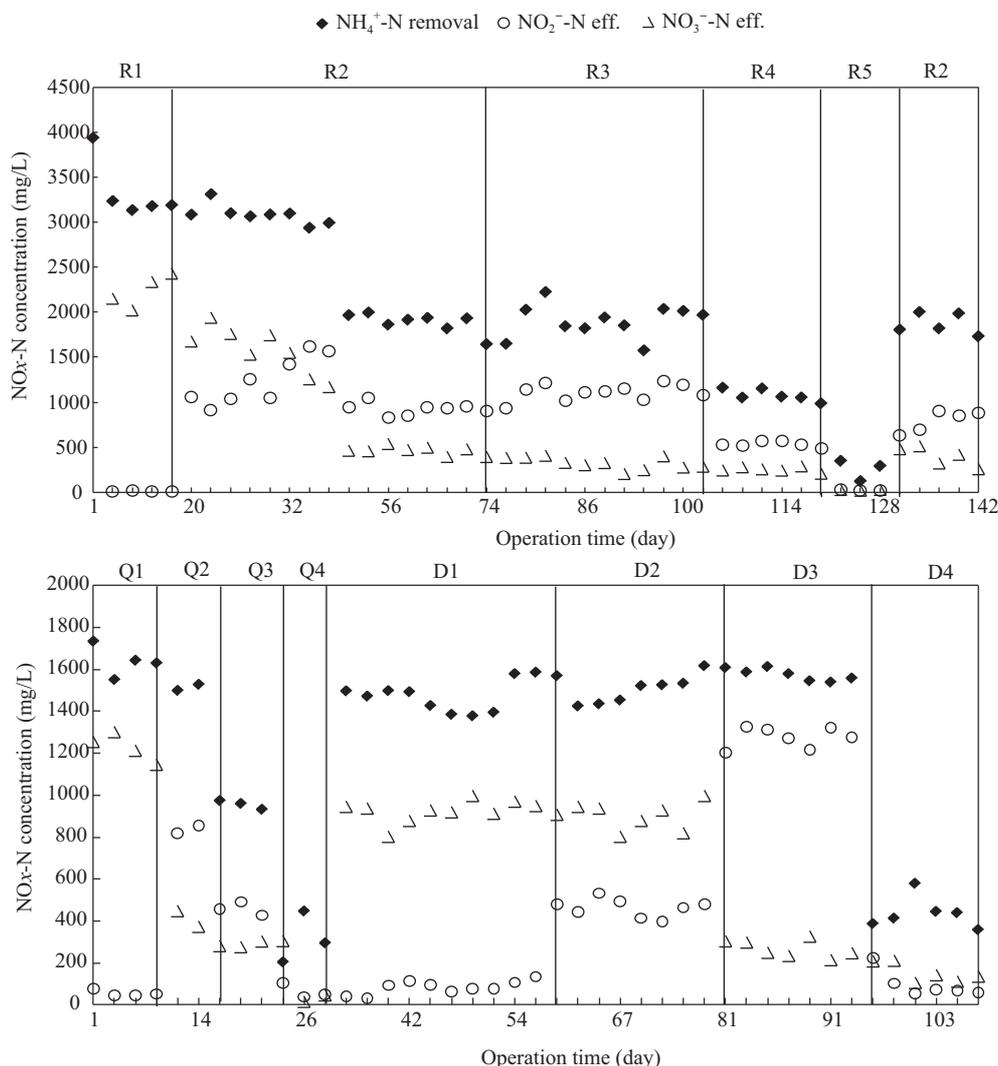
**Fig. 3**  $\text{NH}_4^+$ -N removal and effluent  $\text{NO}_2^-$ -N and  $\text{NO}_3^-$ -N in the reactor. (a) using raw wastewater from Y piggery wastewater treatment plant piggery wastewater treatment plant, (b) using raw wastewater and effluent of anaerobic digester from H piggery wastewater treatment plant.
