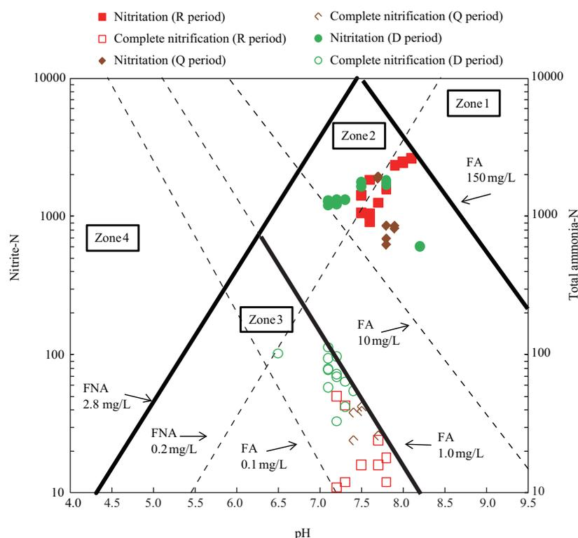
Fig. 5 Inhibition condition graph in the laboratory reactor. FA: free ammonia; FNA: free nitrous acid.
