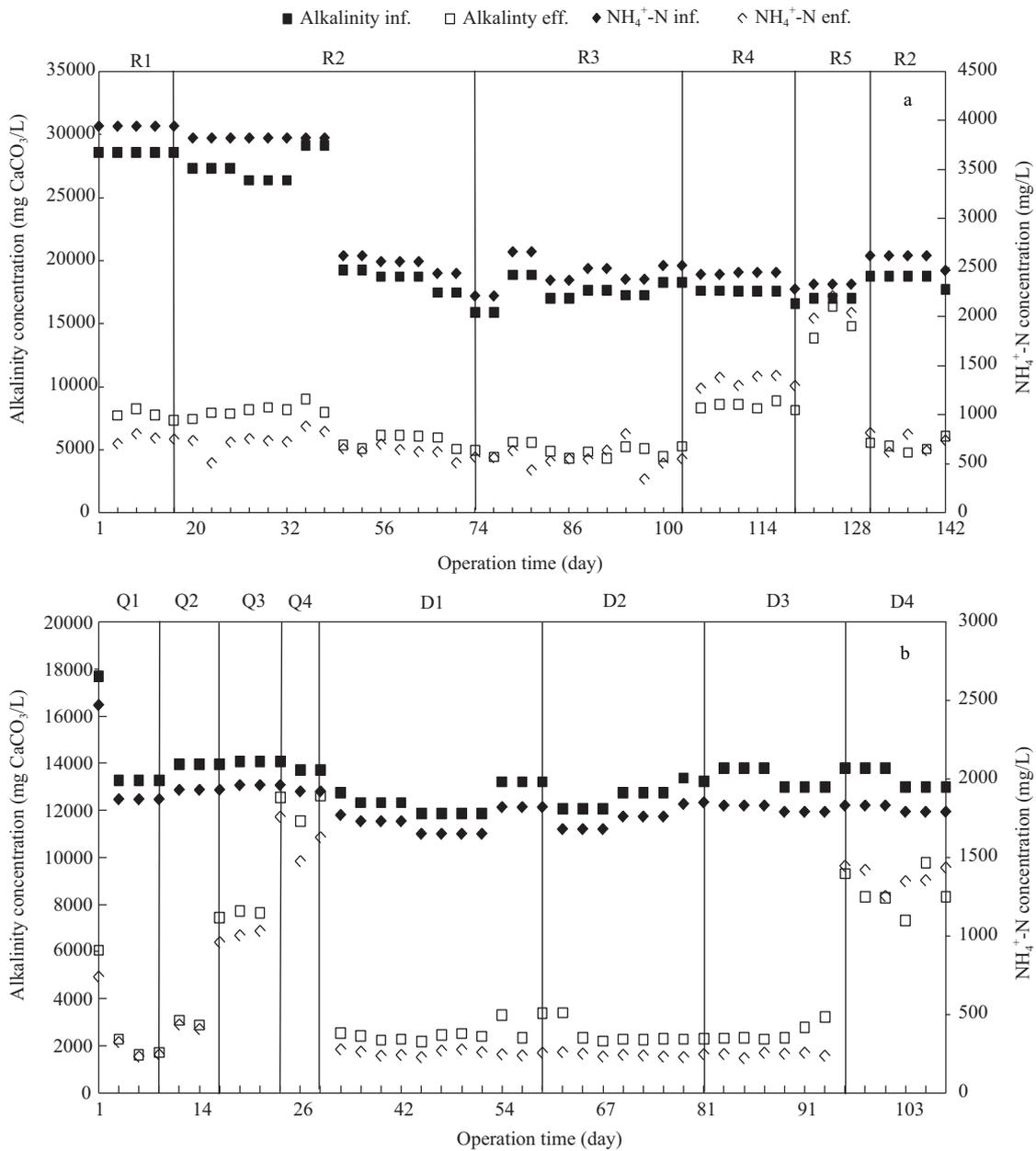
**Fig. 2** Influent and effluent alkalinity and  $\text{NH}_4^+\text{-N}$  in the reactor. (a) using raw wastewater from Y piggery wastewater treatment plant, (b) using raw wastewater and effluent of anaerobic digester from H piggery wastewater treatment plant. The periods of R, Q, and D are referred to Table 2.
