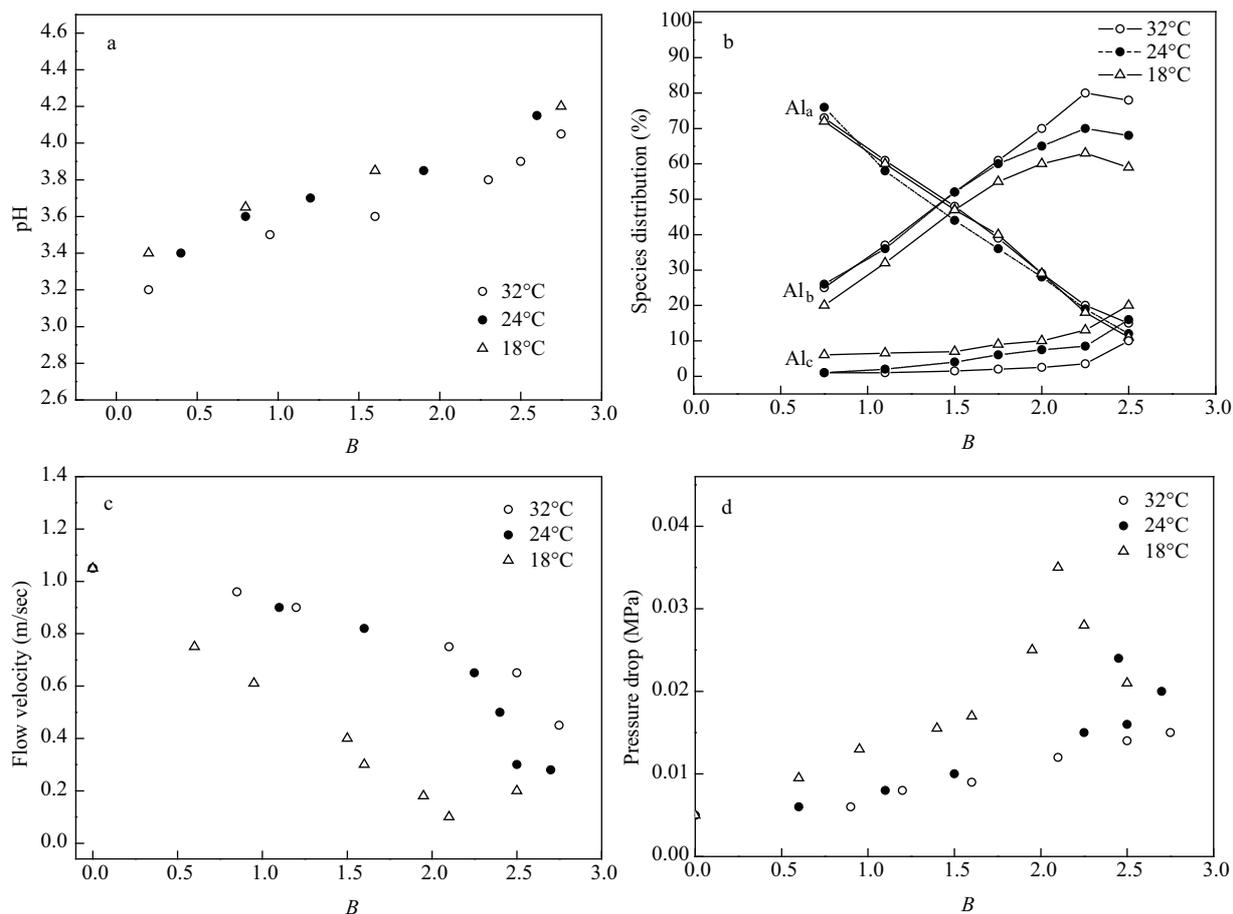
Fig. 2 Evolution of process characteristics with basicity ( $B$ , molar ratio of NaOH to  $\text{AlCl}_3$ ) at different temperatures.
