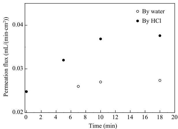
Fig. 5 Recovery of membrane permeation fluxes.
