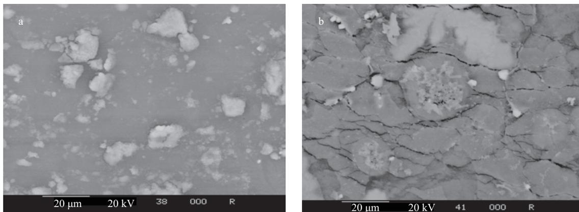
Fig. 4 SEM images of membrane inner surface. (a)  $B = 1.54$ ; (b)  $B = 2.75$ .
