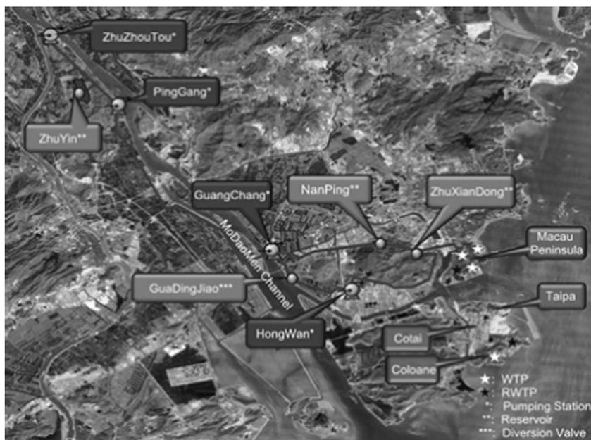
Fig. 1 – Raw water supply system of Macau.
