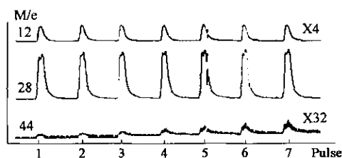
Fig. 6 CO pulse reaction over Au/ZnO (300°C O 2 30 min) catalyst
