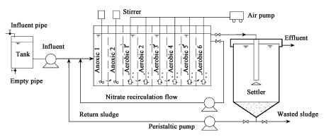
Fig. 1 Schematic diagram of the pilot pre-denitrification process.
