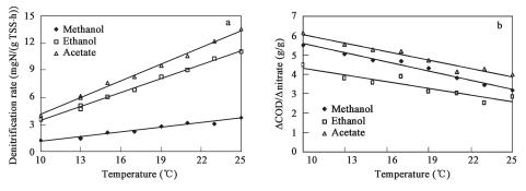
Fig. 3 Denitrification rates (a) and the consumed COD to nitrate-N ratio (b) for different carbon sources.
