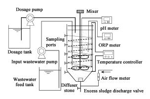
Fig. 2 Schematic diagram of the SBR reactor.
