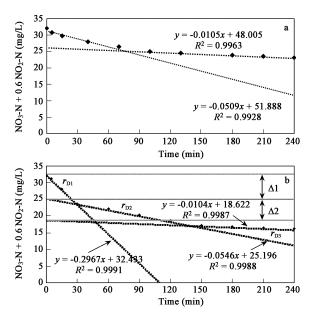
Fig. 4 Typical trend of the nitrate of starch wastewater without (a) and with (b) the waste ethanol addition.
