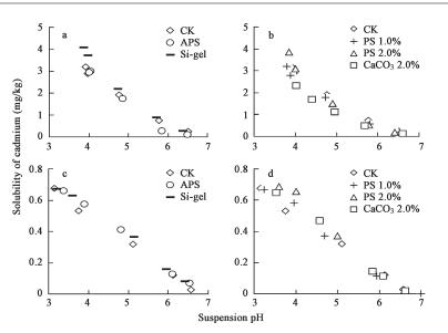
Fig. 2 Solubility of soil cadmium vs. suspension pH. (a) and (b) in Andosol soil; (c) and (d) in Alluvial soil.
