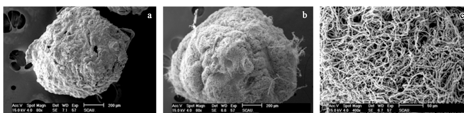
Fig. 6 SEM micrographs of Na-CMC gel beads. (a) Na-CMC plain gel bead ( \times 80 ); (b), (c) Na-CMC immobilized bead ( \times 80 , \times 400 ).
