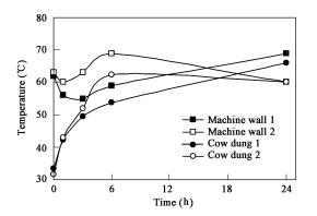
Fig. 2 Temperature change of the machine wall and cow dung during heat treatment.
