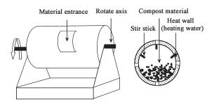
Fig. 1 Assumption diagram of drum rotation heat-treatment machine.
