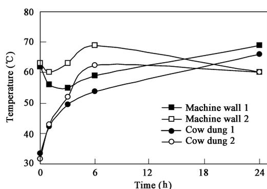
Fig. 2 Temperature change of the machine wall and cow dung during heat treatment.
