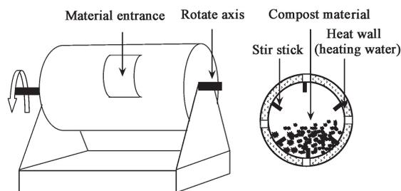
Fig. 1 Assumption diagram of drum rotation heat-treatment machine.
