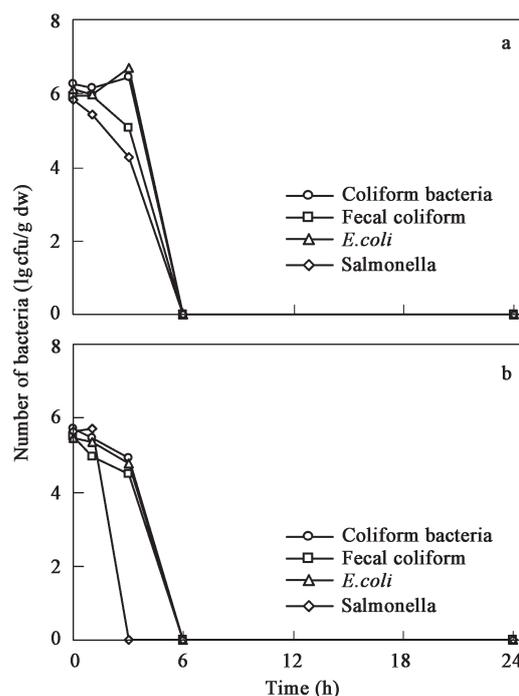
Fig. 3 Number change of pathogenic indicator bacteria during heat treatment. (a) cow dung 1; (b) cow dung 2. not detected ( $<10^2$  cfu/g dw) to coliform bacteria, *E. coli* and salmonella; not detected ( $<10^1$  MPN/g dw) to fecal coliform.
