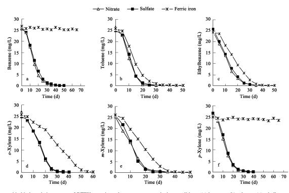
Fig. 1 Anaerobic biodegradation curves of BTEX at various electron acceptor reducing conditions. (a) benzene; (b) toluene; (c) ethylbenzene; (d) *o*-xylene; (e) *m*-xylene; (f) *p*-xylene.
