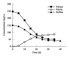
Fig. 2 Curve of nitrate, nitrite and sulfate during anaerobic biodegradation of benzene.
