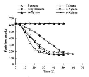
Fig. 3 Curve of Fe<sup>3+</sup> during anaerobic biodegradation of BTEX.
