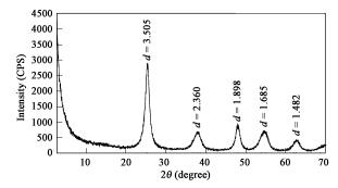
Fig. 3 XRD spectrum of the anatase type nano TiO<sub>2</sub>.
