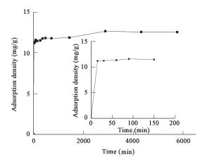
Fig. 5 Adsorption kinetics of Zn(II) on anatase type nano TiO<sub>2</sub>.
