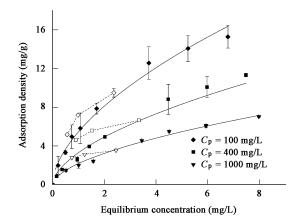
Fig. 6 Adsorption isotherms and their simulating curves under three different  $C_p$  conditions for adsorption of Zn(II) on anatase type nano TiO<sub>2</sub>. Points were experimental data. Lines were modeled results using the MEA-Freundlich-type particle concentration effect isotherm equation. The open symbols were for two-step desorption data.
