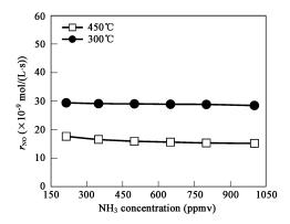
Fig. 2 Effect of NH<sub>3</sub> concentration on the rate of NO conversion at 300 and 450°C. Conditions: catalyst 0.2 g; NO 500 ppmv; O2 6 vol%; total flow rate 300 ml/min.
