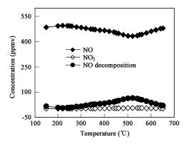
Fig. 4 Effect of temperature on the concentration of NO, NO<sub>2</sub> and the decomposition of NO over Fe-Mo/ZSM-5 catalyst. Conditions: NO 502 ppmv; NO<sub>2</sub> 4 ppmv; O<sub>2</sub> 2 vol%; gas flue rate 300 ml/min.
