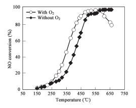
Fig. 1 Change of NO conversion with temperature with 2 vol%  $O_2$  and without O<sub>2</sub>.
