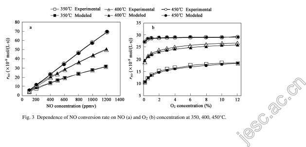
Fig. 3 Dependence of NO conversion rate on NO (a) and O<sub>2</sub> (b) concentration at 350, 400, 450°C.
