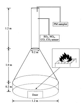
Fig. 1 Schematic diagram of burning tower with sampling attachment.
