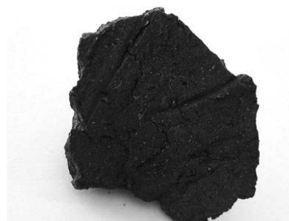
Fig. 2 Photograph of the appearance image of a typical sintered material. Sintering temperature was 400°C.
