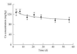
Fig. 4 Concentration of 0.01 mol/L CaCl<sub>2</sub>-extractable Cu in soils aged from 3 to 56 d.
