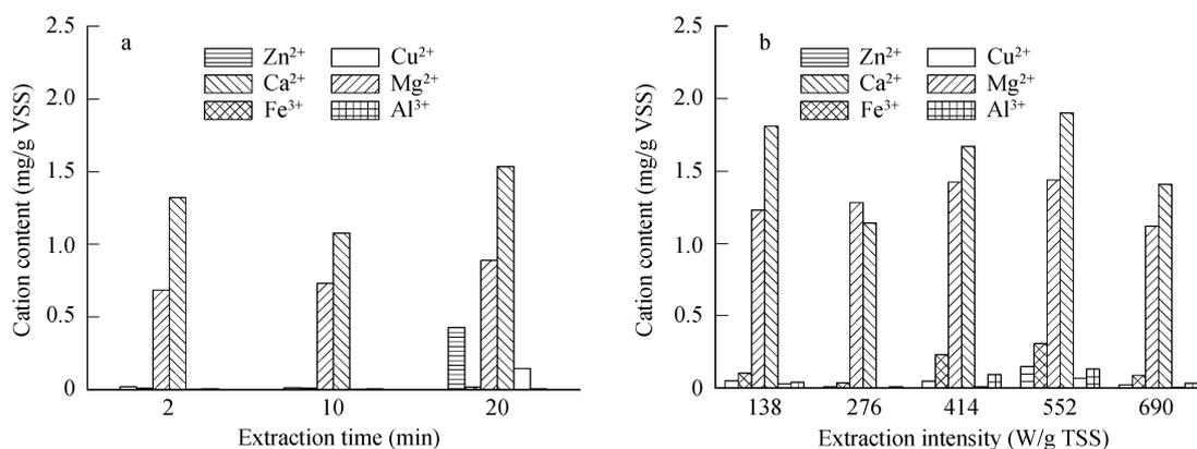
**Fig. 6** Extraction efficiency of cation content with (a) at the level of 138 W/g TSS; (b) at the level of 10 min.
