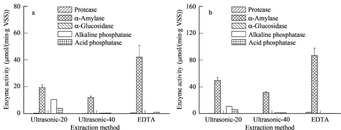
**Fig. 2** Comparisons of extraction methods for sludge flocs from (a) aerated basin and (b) returned sludge (error bars represent standard deviation).
