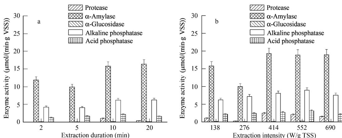
**Fig. 4** Enzyme extraction efficiency of sludge flocs from aerated basin (error bars represent standard deviation). (a) at the level of 138 W/g TSS; (b) at the level of 10 min.
