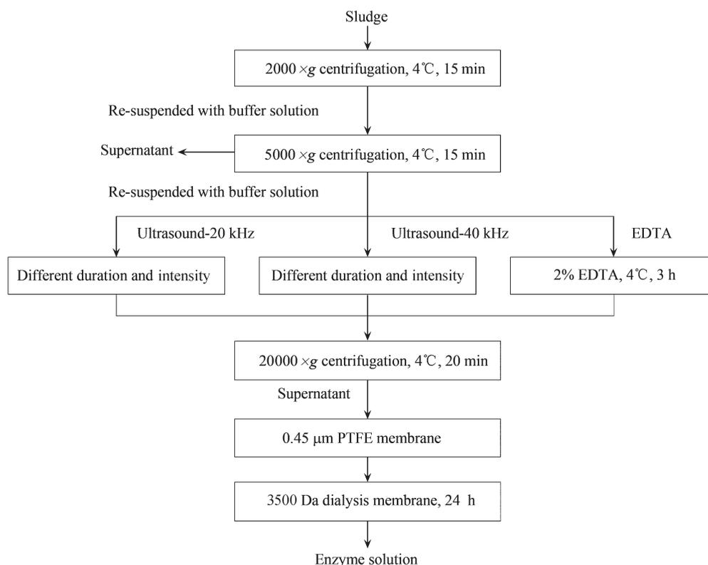
**Fig. 1** Enzymes extraction protocol from sludge flocs.
