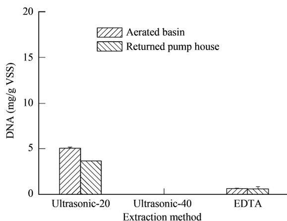
**Fig. 3** Comparisons of extraction method on DNA extraction efficiency (error bars represent standard deviation).
