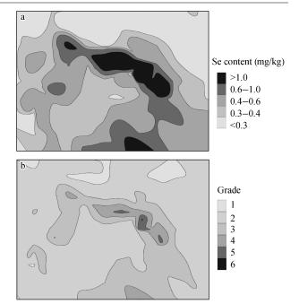
Fig. 3 Spatial distribution of Se content (a) and contamination (b) in agricultural soils by geostatistical interpolation using MapGis.
