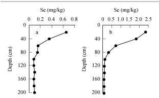
**Fig. 2** Variation in Se concentrations with soil profiles in cropland (a) and a site beside a power plant (b).
