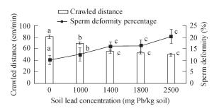
**Fig. 1** Mean  $(\pm SD)$  crawled distance in one minute on day 7 and mean  $(\pm SD)$  of sperm deformity percentage (%) on day 14. Identical letters indicate statistically identical values.
