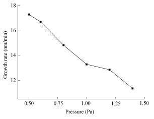
Fig. 1 Growth rate at different working pressures.
