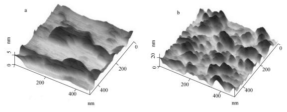
Fig. 6 Atomic force microscopy (AFM) morphological images of TiO<sub>2</sub> films deposited at 0.4 Pa (a) and 1.4 Pa (b).
