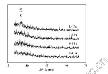
Fig. 2 X-ray diffraction (XRD) patterns of TiO<sub>2</sub> films deposited at different working pressures.
