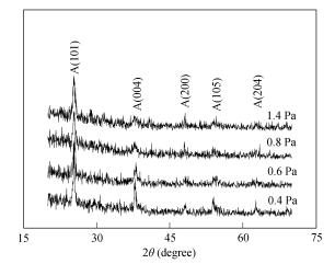
Fig. 4 XRD patterns of  $TiO_2$  films after thermal annealing treatment at 500°C.
