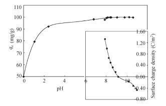
**Fig. 1** Adsorption of MB onto Florisil 200  $\mu$ m  $d_p$ ,  $C_0 = 1000$  mg/L, 24 hr, 20°C, and the surface charge density as a function of pH.
