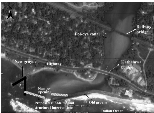
Fig. 6 Satellite image of lagoon mouth with proposed structural intervention with respect to existing structures.
