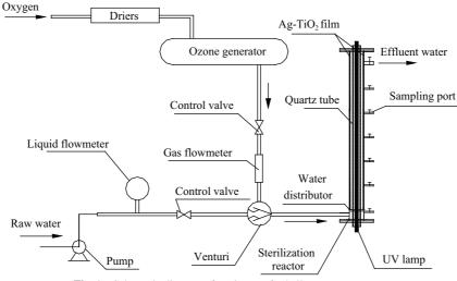
Fig. 1 Schematic diagram of equipment for ballast water treatment.
