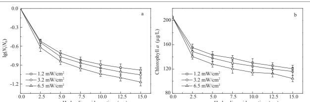
Hydraulic residence time (sec)Hydraulic residence time (sec)Fig. 4Effect of UV intensity on D. salina inactivation in UV/Ag-TiO<sub>2</sub>/O<sub>3</sub> system. (a) inactivation efficiency; (b) chl-a removal efficiency (ozone dose= 0.36 g/hr; temperature = 20°C).
