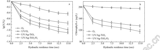
**Fig. 2** Comparison of the inactivation of *D. salina* using the combined UV/Ag-TiO<sub>2</sub>/O<sub>3</sub> process with that in individual unit processes. (a) inactivation efficiency; (b) chl-*a* removal efficiency (UV intensity =  $3.2 \text{ mW/cm}^2$ ; ozone dose = 0.36 g/hr; temperature =  $20^{\circ}$ C).
