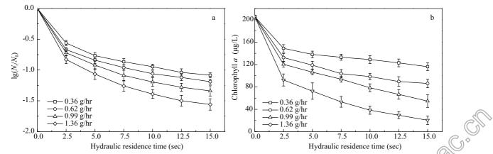
Fig. 3 Effect of ozone dose on *D. salina* inactivation in UV/Ag-TiO<sub>2</sub>/O<sub>3</sub> system. (a) inactivation efficiency; (b) chl-*a* removal efficiency (UV intensity =  $3.2 \text{ mW/cm}^2$ ; temperature =  $20^{\circ}$ C).
