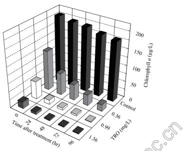
**Fig. 5** Decay of *D. salina* and chl-*a* in the effluent of UV/Ag-TiO<sub>2</sub>O<sub>3</sub> process at 20°C.
