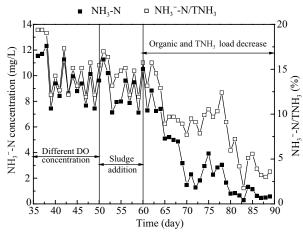
Fig. 6 NH<sub>3</sub>-N concentration and ratio of NH<sub>3</sub>-N/TNH<sub>3</sub> during the period of nitrification recovery.
