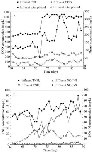
**Fig. 5** COD and total phenol removal (a) and TNH<sub>3</sub> removal (b) of the MBBR after adding more dilute water into the influent.
