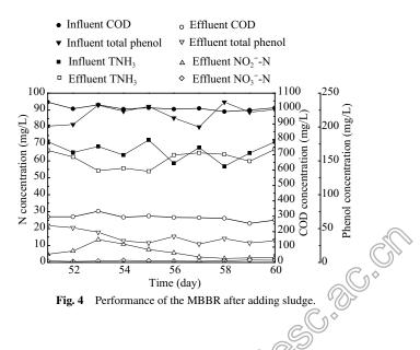
Nitrification of the MBBR was improved after adding nitrifying sludge and effluent  $NO_2^{-}-N$  concentration reached 15 mg/L at day 53, but decreased gradually and almost ceased at day 58 (Fig. 4). The sludge adding into the MBBR was cultured in a batch manner which would promote nitrifying bacteria growing. That was the reason why nitrification of the system recovered partly after adding nitrifying sludge. COD and total phenol removal
