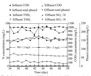
Fig. 3 Performance of the MBBR after increasing DO concentration in the bulk liquid.
