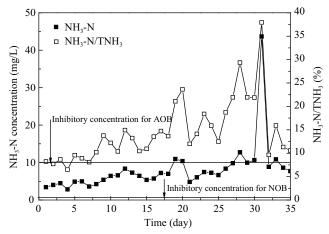
**Fig. 2** NH<sub>3</sub>-N concentration and ratio of NH<sub>3</sub>-N/TNH<sub>3</sub> before and after nitrification inhibition.
