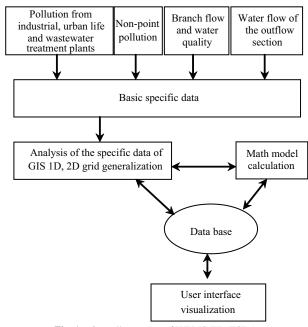
Fig. 1 Overall structure of WPMS\_ER\_TGRA.
