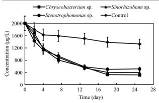
Fig. 2 Degradation of geosmin (2 mg/L). Error bars represent the standard deviation of triplicate observations.
