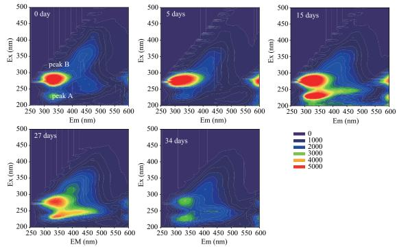
Fig. 5 Fluorescence EEM of the LB-EPS fraction for sonicated sludge.
