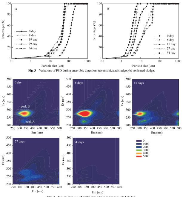
Fig. 4 Fluorescence EEM of the slime fraction for sonicated sludge.
