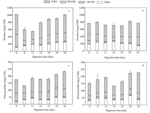
Fig. 2 Evolutions of organic matters during anaerobic digestion. (a) proteins for unsonicated sludge; (b) proteins for sonicated sludge; (c) polysaccharides for unsonicated sludge; (d) polysaccharides for sonicated sludge.
