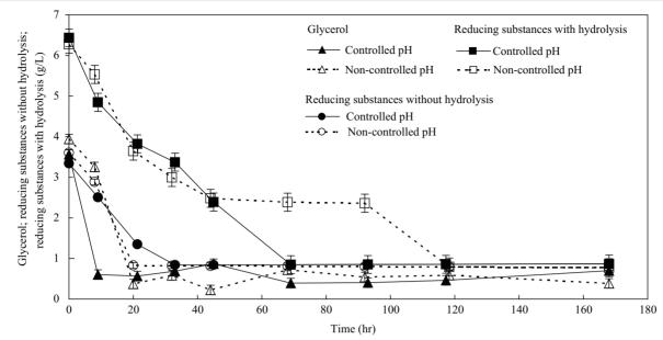
Fig. 4 Variations in the concentrations of glycerol and reducing substances in beet molasses vinasse during STR processes with and without pH control. The length of each error bar is twice the standard deviation of the measured concentration (n = 3).
