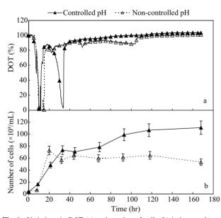
Fig. 1 Variations in DOT (a) and number of cells (b) in beet molasses vinasse during STR (stirred-tank reactor) processes with and without pH control. The length of each error bar is twice the standard deviation of the measured concentration (n = 3).
