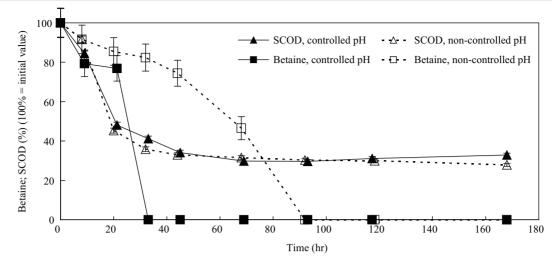
Fig. 2 Variations in SCOD and betaine concentration in beet molasses vinasse during STR processes with and without pH control. The length of each error bar is twice the standard deviation of the measured concentration (n = 3).
