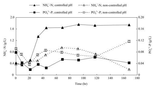
Fig. 3 Variations in ammonia and phosphate concentrations in beet molasses vinasse during STR processes with and without pH control. The length of each error bar is twice the standard deviation of the measured concentration (n = 3).
