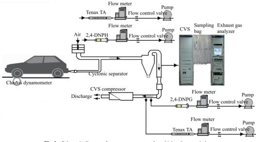
Fig. 1 Schematic diagram of measurement system for vehicle exhaust emissions.
