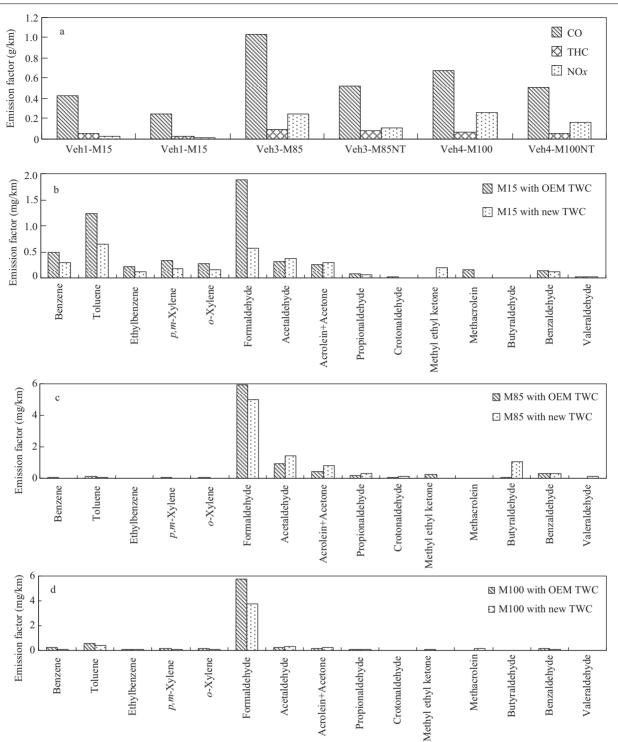
Fig. 3 Regulated emissions, BTEX and carbonyls comparison between OEM TWC and new TWC for M15, M85 and M100 respectively. (a) regulated emissions; (b) M15; (c) M85; (d) M100.
