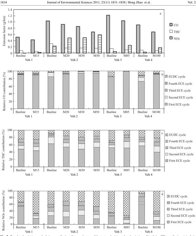
Fig. 2 Regulated emissions and relative contributions from each stage of the test cycle. (a) regulated emissions; (b) relative CO contribution; (c) relative THC contribution; (d) relative NOx contribution.
