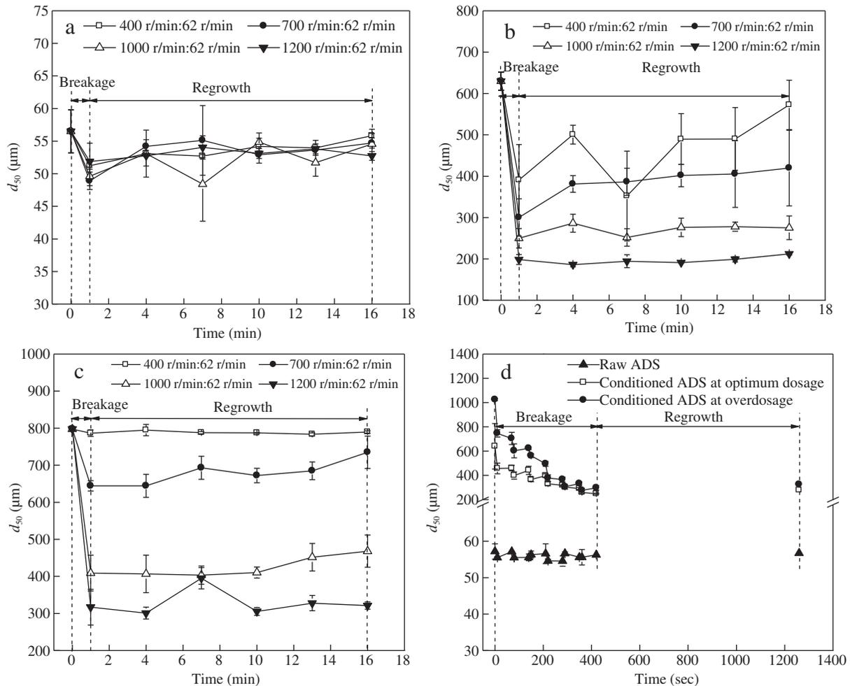
**Fig. 2 – Change in the floc size ( $d_{50}$ ) of ADS with time under different shear modes. (a) Raw ADS, (b) optimum dosage-conditioned ADS, (c) overdosage-conditioned ADS under CSS-SR mode, and (d) raw and conditioned ADS under MPS-SR mode.**
