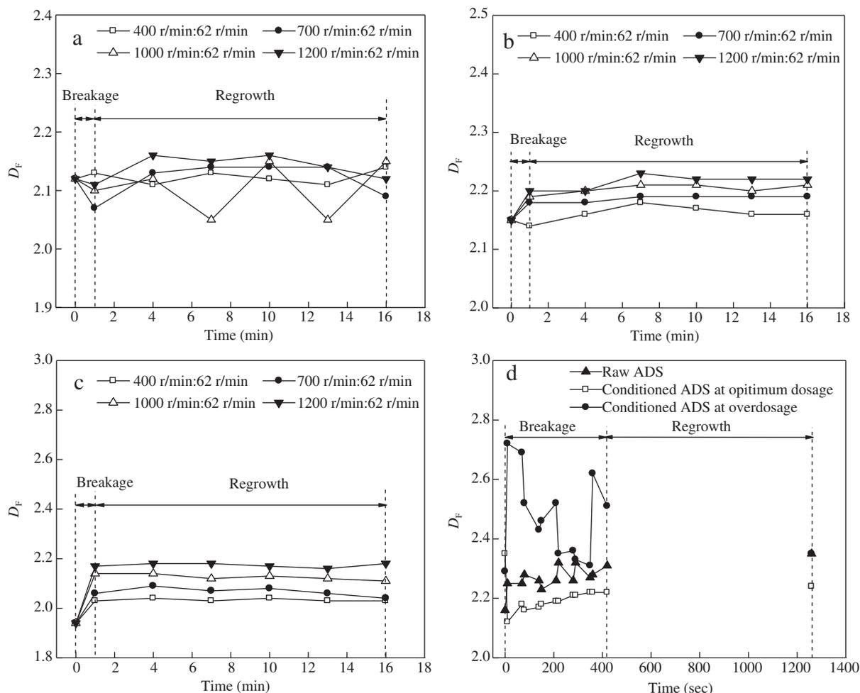
**Fig. 3 – Change in the fractal dimension of ADS with time under different shear modes.(a) Raw ADS, (b) optimum dosage-conditioned ADS, (c) overdosage-conditioned ADS under CSS–SR mode, and (d) raw and conditioned ADS under MPS–SR mode.**
