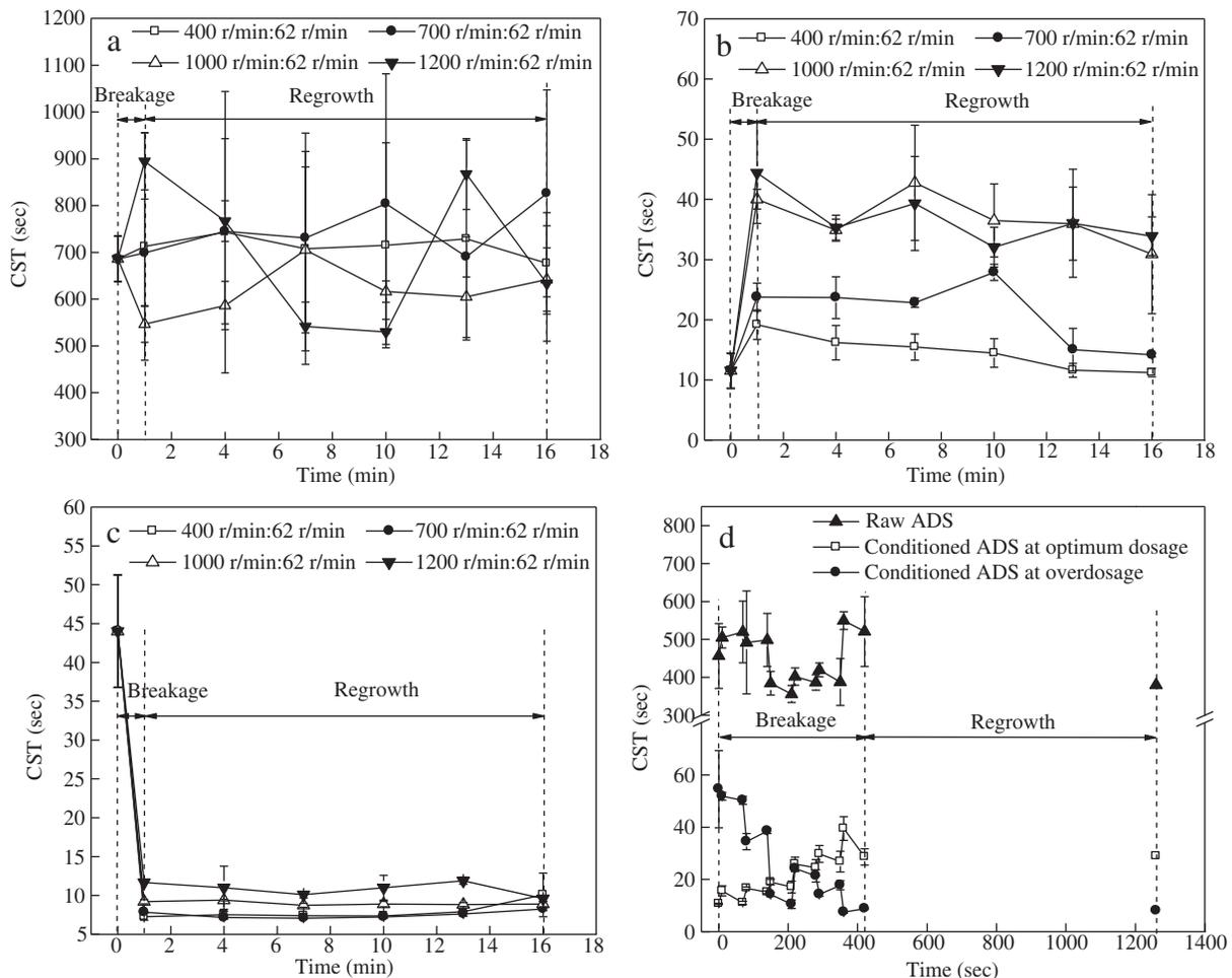
Fig. 4 – Changes in CST of ADS with time under different shear modes. (a) Raw ADS, (b) optimum dosage-conditioned ADS, (c) overdosage-conditioned ADS under CSS-SR mode, and (d) raw and conditioned ADS under MPS-SR mode.
