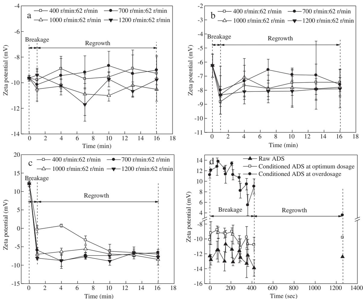
**Fig. 1 – Changes in the zeta potential of anaerobic digested sludge (ADS) with time under different shear modes. (a) Raw ADS, (b) optimum dosage-conditioned ADS, (c) overdosage-conditioned ADS under the continuous strong shear (CSS)-self-regrowth (SR) mode, and (d) raw and conditioned ADS under the multipulse shear (MPS)-SR mode.**
