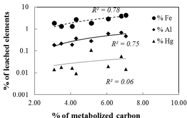
**Fig. 4 – Percentage of leached metals (Fe, Al, Hg) versus percentage of metabolized carbon (amount of organic acids produced normalized at consumed carbon sources) on day 10.**
