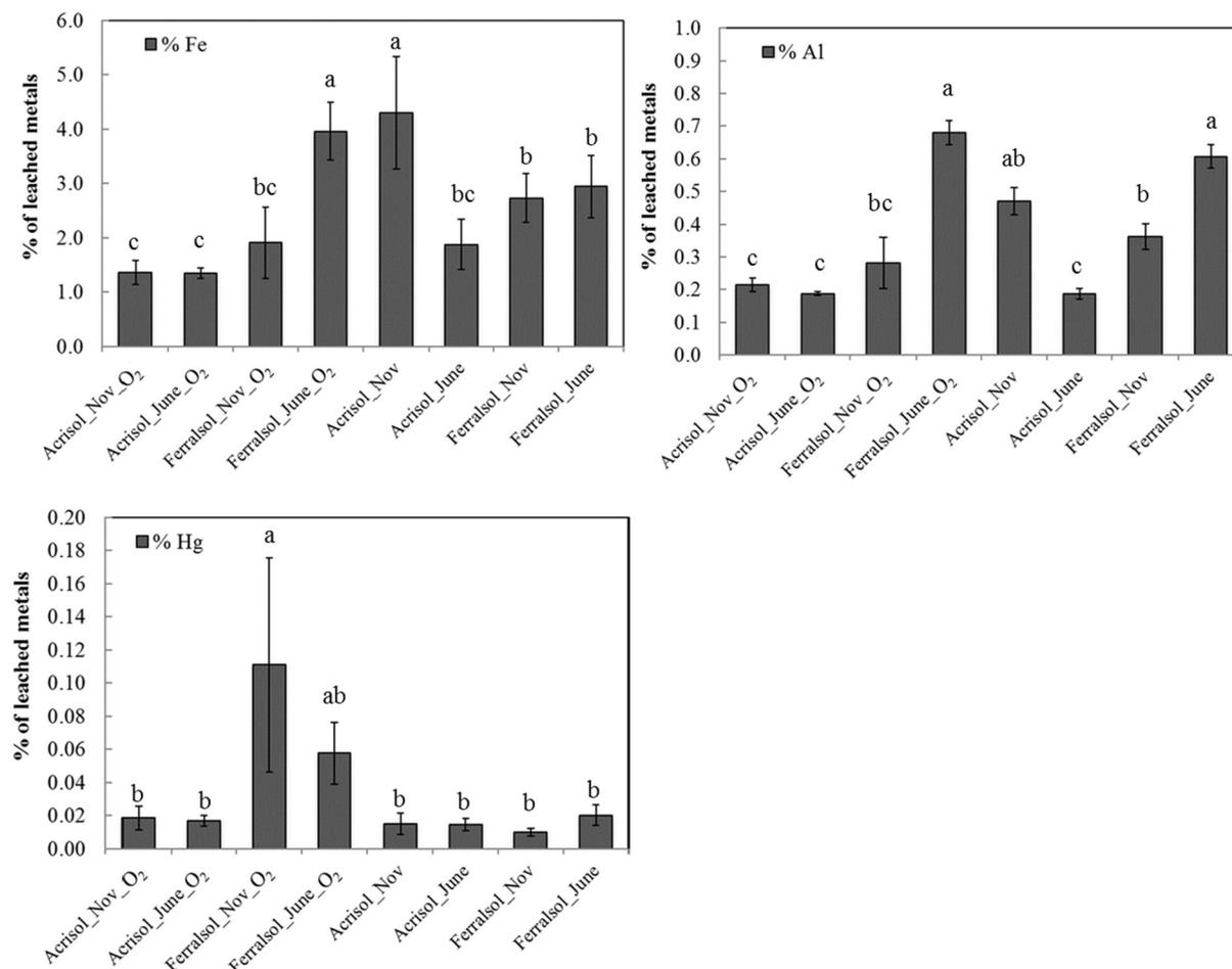
**Fig. 3 – Percentage of leached metals (Fe, Al, Hg) at the end of cinnabar ore biodissolution experiments. Each bar represents the mean and standard deviation calculated from three replicates. The symbols a, b, c and d correspond to the different groups of significance obtained by analysis of variance and by the Tukey test ( $p = 0.05$ ) on three replicates.**
